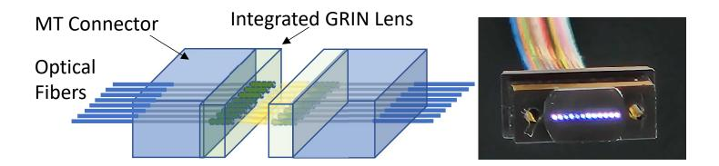
EB-MT connectors with GRIN lens can operate even in the liquid coolant, dust-free and bubble-free, easy to cleaning, low stress, without MPO housing.
